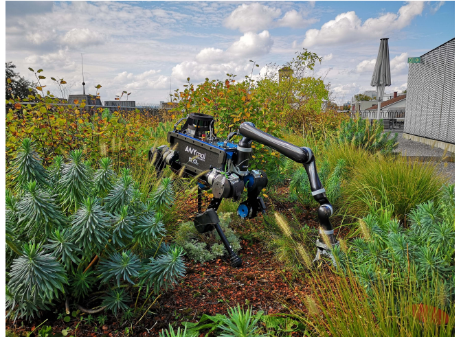
Fig. 1. The quadrupedal robot ANYmal equipped with a six DOF robotic arm. The system is fully torque-controlled, enabling compliant behavior and safe interaction.
